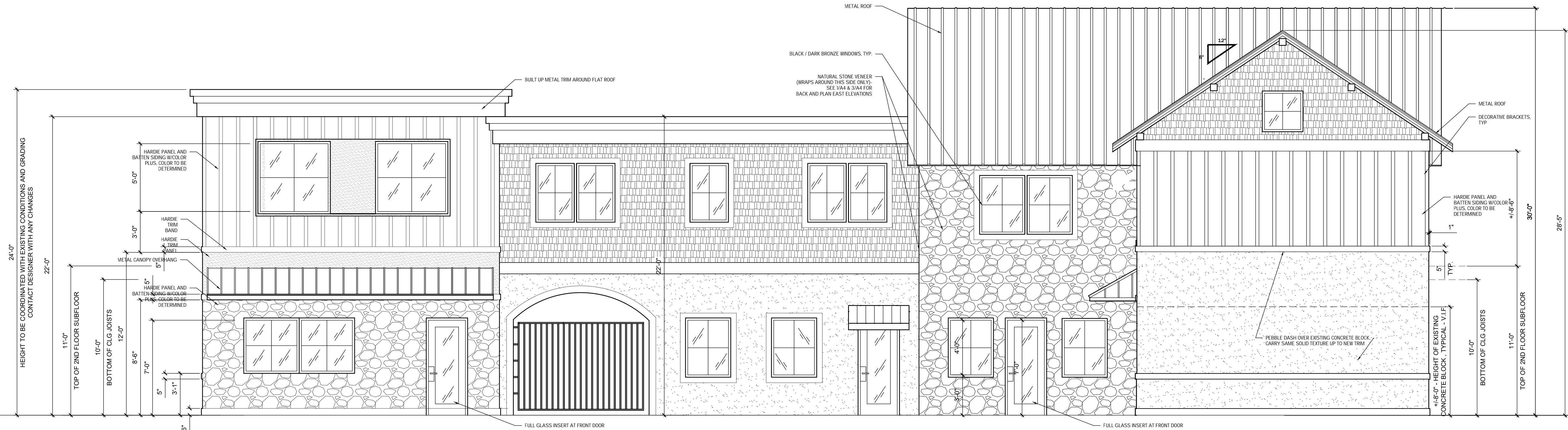
FRONT ELEVATION - BUILDING 3R - (BUSINESS) SCALE: 1/4"=1'-0" 1-A3
