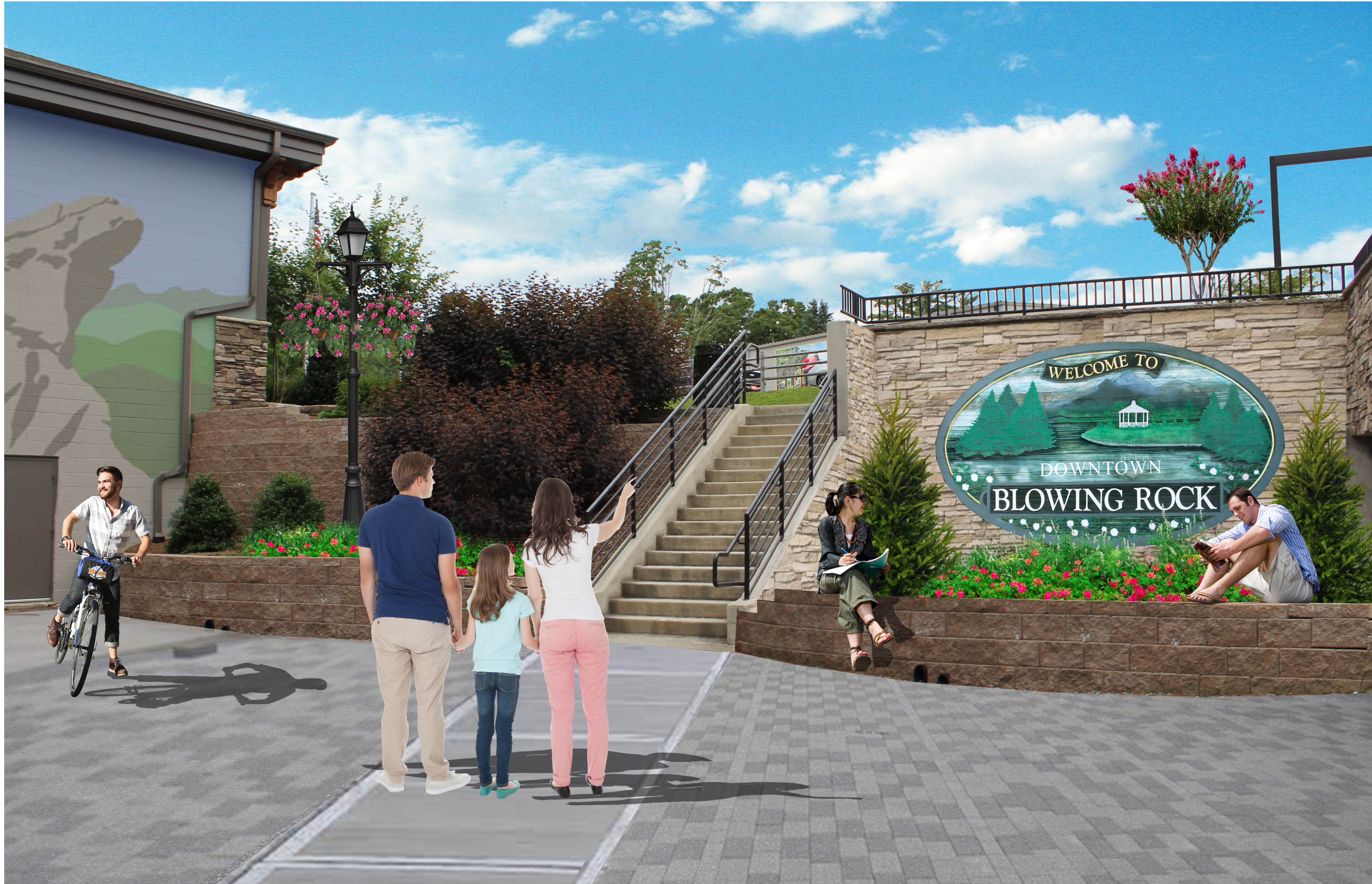
The service area of the American Legion building is converted into a pedestrian friendly space with a dedicated crossing, seating walls, plantings, and signage. The asphalt is replaced with pavers and concrete, while still allowing service vehicles to access the bottom floor of the American Legion building.
