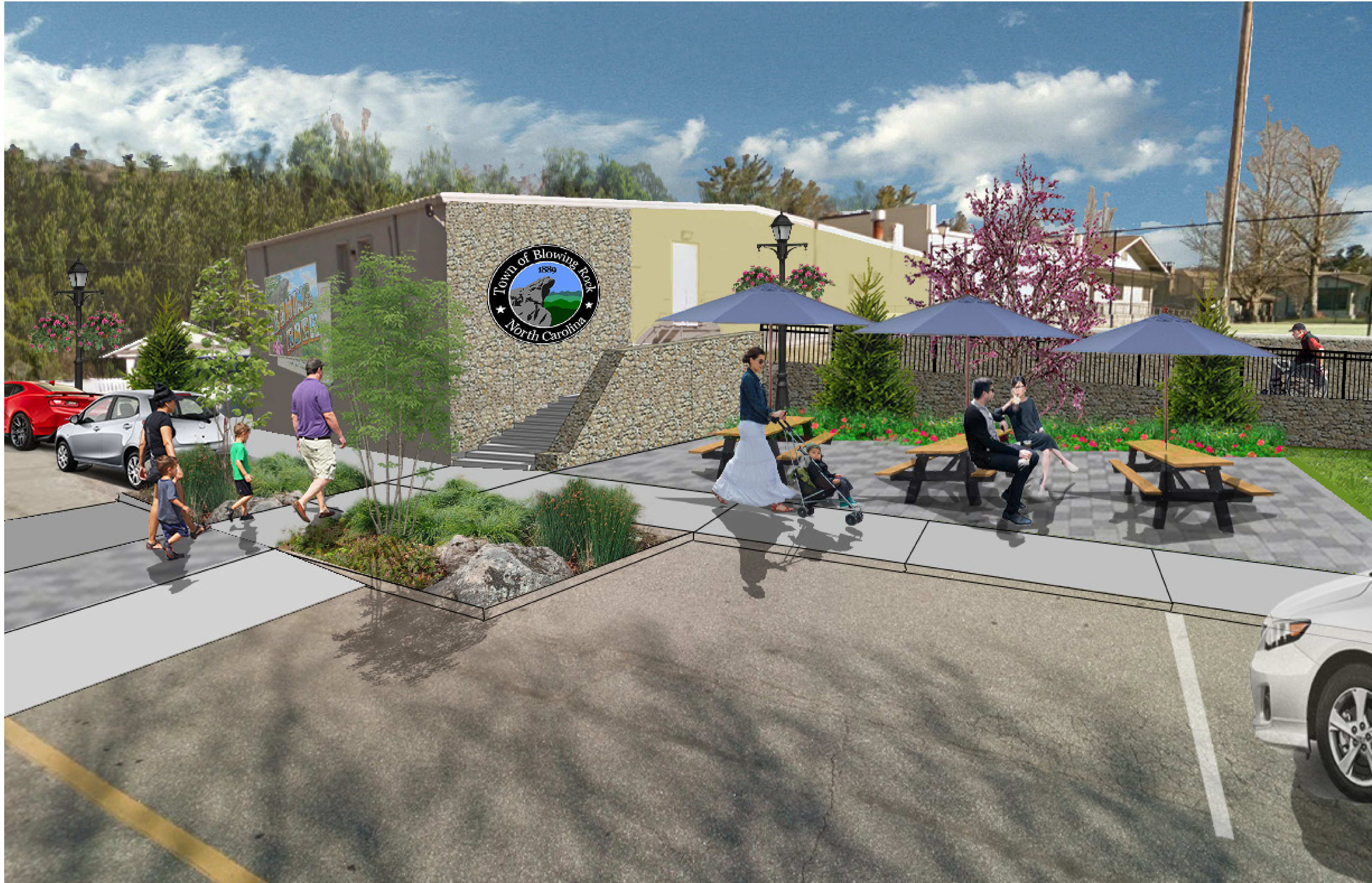
Wallingford Road parking is reorganized into parallel parking with rain garden planters to slow vehicular traffic in an area of heavy pedestrian traffic. The crosswalk serves as a speed bump to slow down traffic and to create a more ADA-friendly crossing. The plaza serves as a place for picnicking and social gathering along the street.
