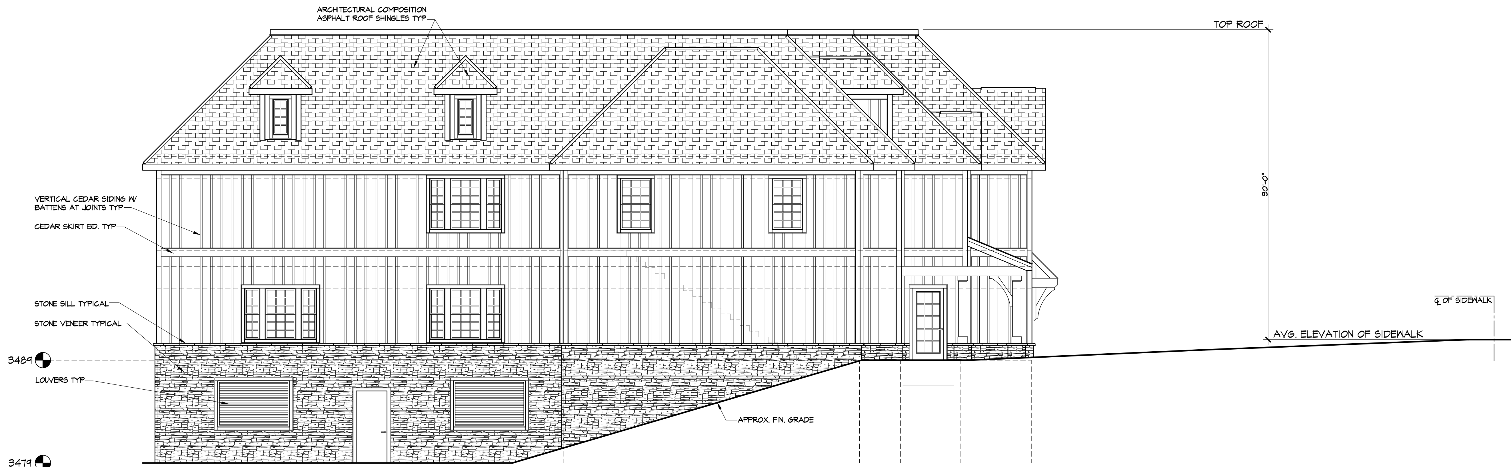
LEFT SIDE ELEVATION SCALE : 3/16" = 1'-0"
